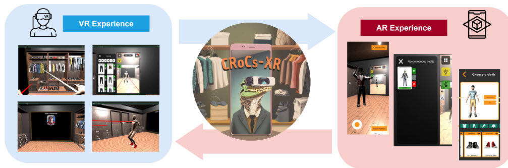
Figure 1: CROCs-XR enables users in Virtual Reality to try on 3D dresses on their avatars, while Users in the physical realm can synchronously visualize, in Augmented Reality, what the user is doing and communicate with her/him through video and audio streaming.
